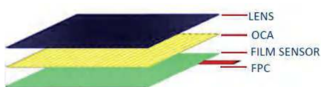
Film Sensor CTP G/F Structure, G/FF Structure
