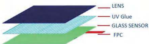
Glass Sensor CTP G/G Structure
